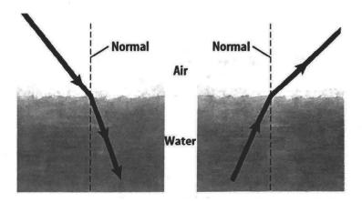
**Wave Speed** The figures above show how a light wave bends when it passes from air to water and water to air. A line that is perpendicular to the water's surface is called the normal. A light ray slows down and bends toward the normal when it passes from air into water. A light ray speeds up and bends away from the normal when it passes from water into air. If the speed of the wave changes a lot between mediums, the direction of the wave will change a lot too.
